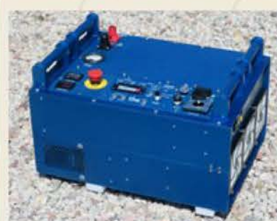
Figure 2. System for shallow and deep ERT (DERT). New transmitting and receiving systems for DERT measurements.
