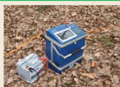
Figure 1. New Syscal Terra system for the Electrical Resistivity Tomography (ERT).
