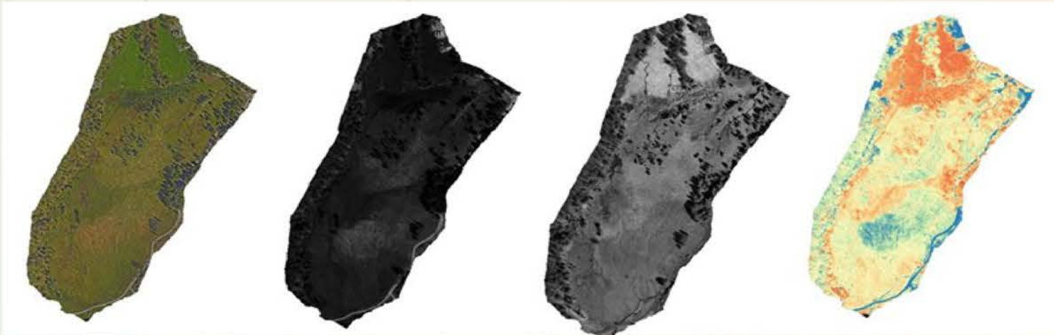
Example: orthophoto-multispectral sequence (low-resolution RGB, RED, NIR, and NDVI)
