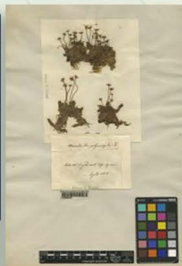
The digitising station for bidimensional herbarium specimen: scanner HerbScan; colorchecker Calibrite and scalebar.
