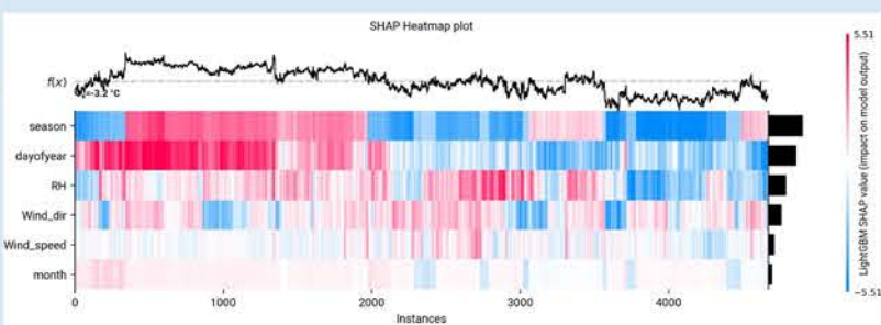
Fig. 6: Heatmap of SHAP values of LightGBM model. The heatmap displays the contribution of each feature to the model's predictions, with positive contributions represented by red cells and negative contributions by blue cells. Colour intensity denotes the magnitude of the contribution. The output of the model, f(x) , is shown above the heatmap matrix, centred around the explanation's base value ( \phi_0 ), and the global importance of each model input is shown in the bar plot on the right-hand side of the plot.
