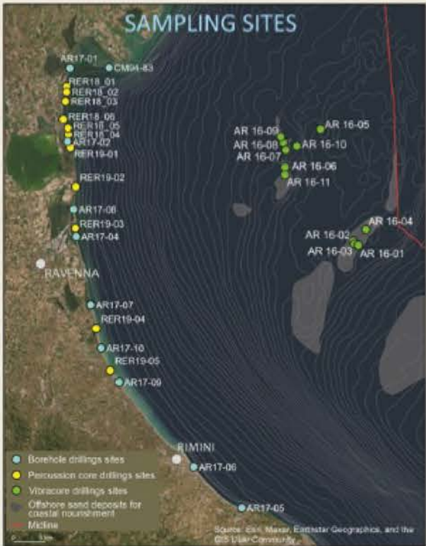
Figure 1 - Study area, showing the sampling locations and three types of sampling methods: 1- Borehole drillings (11 sites); 2- Percussion core drillings (10 sites); 3- Vibracore drillings (10 sites).
