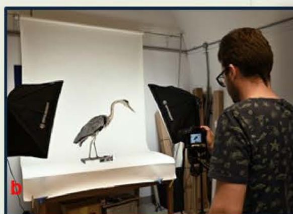
The digitising station for invertebrates (a) and vertebrates (b): camera Nikon z50 with Nikkor ZDX18-140 (a, b); photostand (a); tripod (b); softbox Bresser Daylight set (a, b); colorchecker Calibrite and scalebar (a, b).
