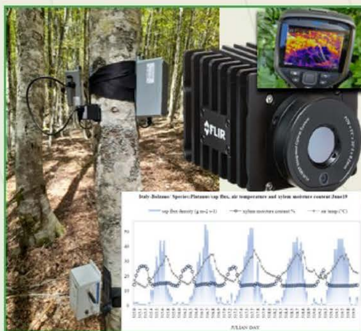
Figure 3. Tree Talker and Thermal camera that will be used in the study sites. Graph shows an example of sap flux, stem humidity and air temperature in hourly scale.
