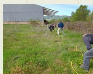
Figure 4. Acquisition of geoelectrical data in one of the test sites of ITINERIS project (Tito industrial areas, Basilicata Region).
