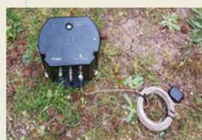
Figure 3. A Triton Accelerometer for analysis of near-surface-soil-infrastructure dynamical interactions and microzonation studies. One of the activities will be focused to integrate geoelectrical and seismic measurements.
