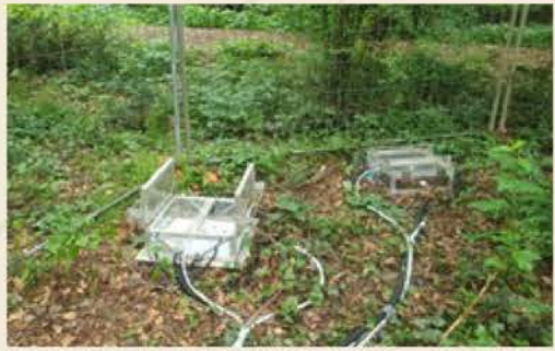
Figure 2: Automatic dynamic chamber system, constructed following the Butterbach-Bahl et al. (2002) design. This system measures surface fluxes of O 3 , NO, NO 2 , and CO 2 and it includes 5 measurement chambers and 1 blank chamber.
