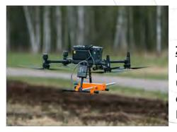
**Zond Aero LF:** drone based ultralight ground penetrating radar system equipped with 3 unshielded dipole antennas working at 3 different central frequencies: 100 MHz, 150 MHz, 300 MHz.
