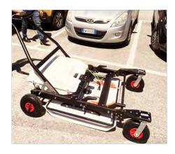
Geoscope MkIV equipped with the array ground coupled G0908: multi-channel multi-frequency ground penetrating radar (GPR) for high-density 3D data capturing. Thanks to the step-frequency technology, the system enables optimal penetration and highest resolution simultaneously by sweeping through a wide frequency range (40 MHz – 3GHz) with only one single antenna array.
