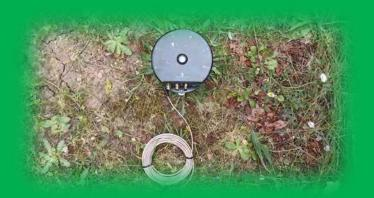
Seismic array consisting of 11 accelerometers, 35 0.5 Hz velocimeters and a nodal system of 60 4.5 Hz 3C geophones for the analysis of the near surface – infrastructure interactions, microzonation studies and microseismic monitoring.
