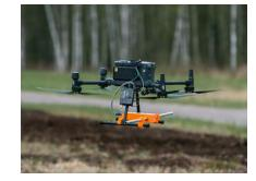
The GPR method allows the detection of the electric permittivity contrasts.
