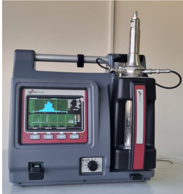
Figure 1. Instruments for online measurements of aerosol properties available at CIAO and purchased within ITINERIS: a) 14-stage cascade impactor; b) total carbon analyzer (on the left) and ethalometer (on the right); c) APS.
