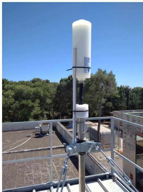
Figure 11. Setup with HEPA filter for TOF-ACSM.
