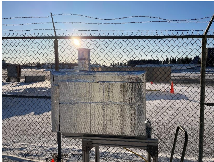
Figure 5 FIRMOS measuring atmospheric zenith-sky IR spectra at Ottawa airport.
