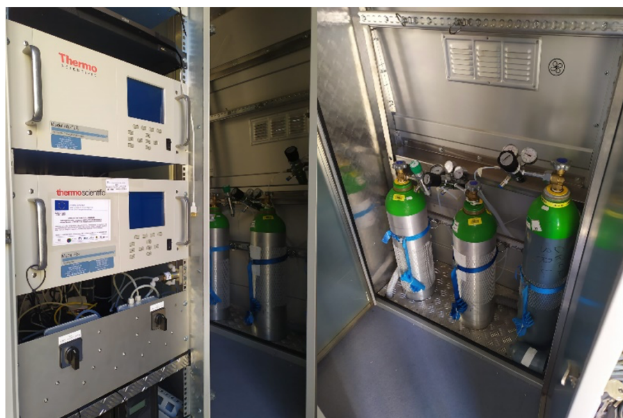
Figure 8: Picture of the calibration system installed and operative in the MAGA exploratory platform.
