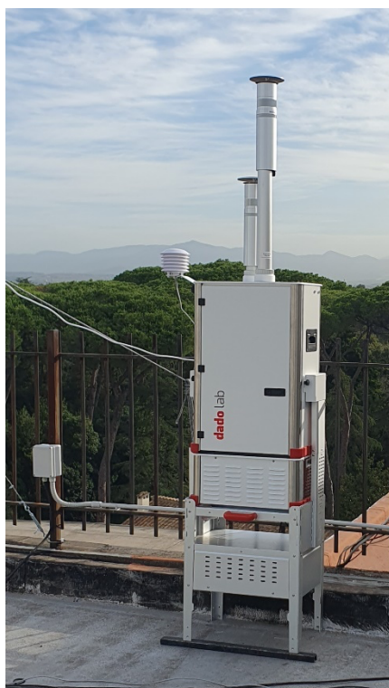
Figure 9: Dual Channel sampler with eBC measurements installed in Rome for a measurement campaign during autumn 2024.
