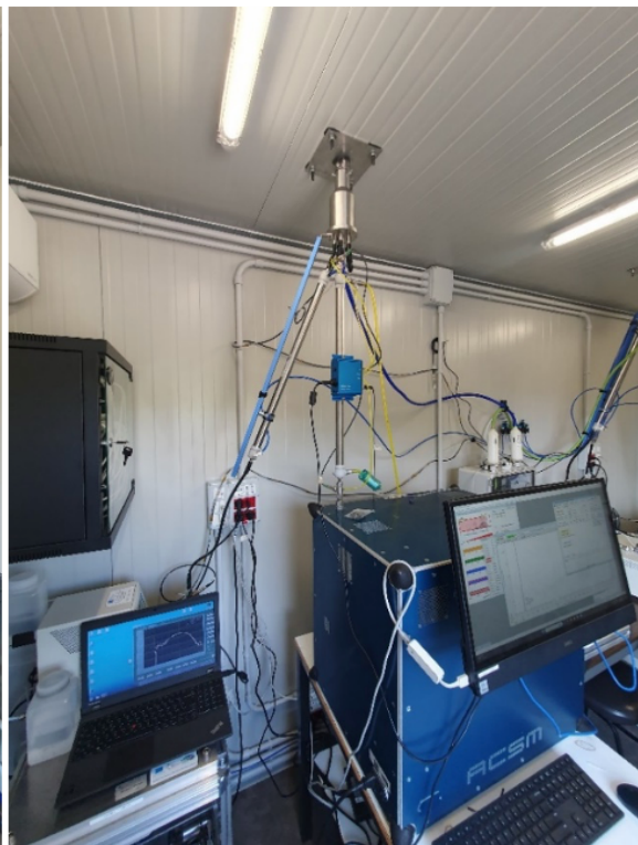
Figure 13: Pictures of the interior of the new shelter and details of the PM10 and PM2.5 inlets.
