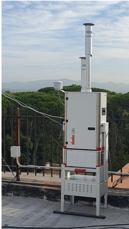
Figure 12: Dual Channel sampler with eBC measurements installed in Rome for a measurement campaign during autumn 2024.
