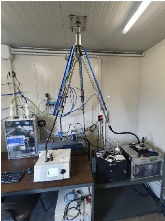
Figure 20: Pictures of the interior of the new shelter and details of the PM10 and PM2.5 inlets.
