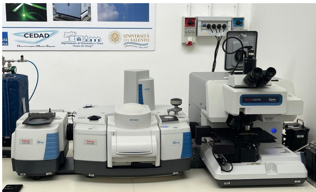
Figure 6: The Thermo Fisher Scientific Nicolet iS50 FTIR system.
