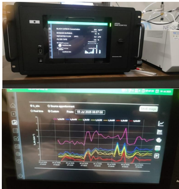
Figure 13: Aethalometer AE36 operating at the ACTRIS site in Lecce.
