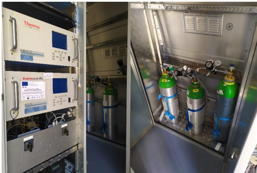
Figure 11: Picture of the calibration system installed and operative in the MAGA exploratory platform.
