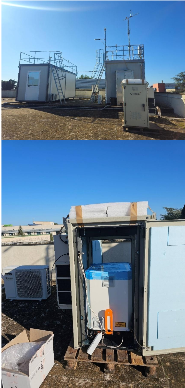
Figure 23: View of the LIDAR system installed on rooftop of CNR-ISAC Lecce building.
