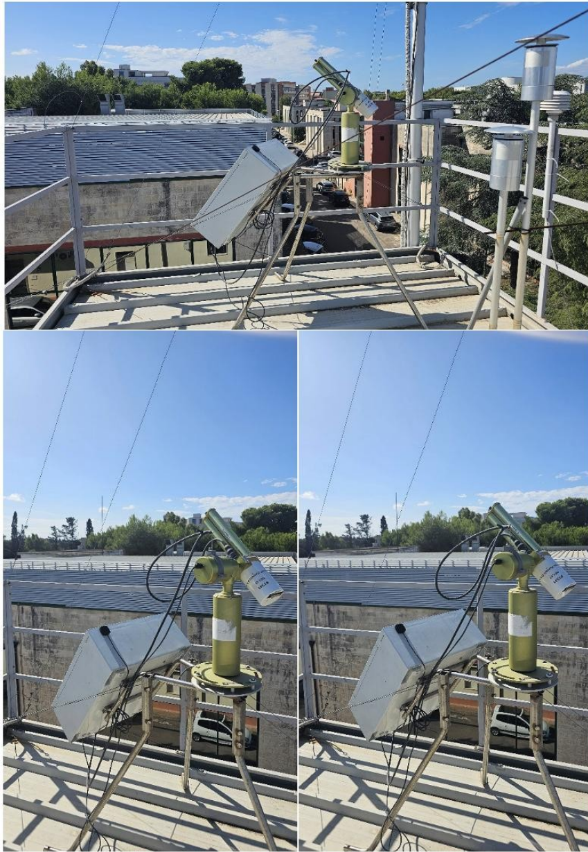
Figure 22: View of the Sun/sky/lunar photometer CIMEL CE318-T located on rooftop of CNR-ISAC Lecce building
