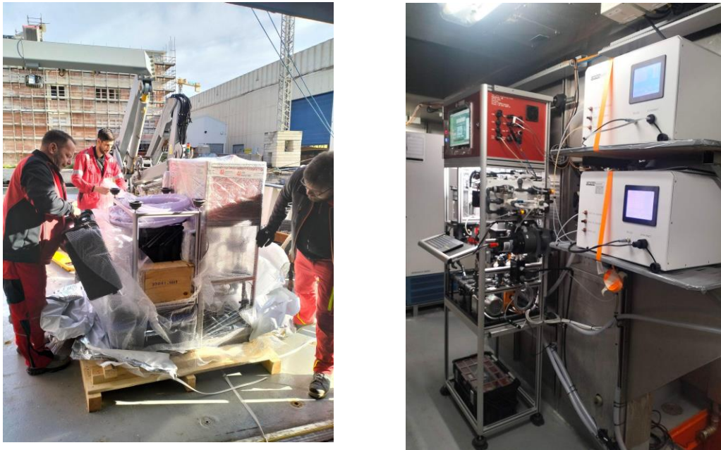
Figure 1. FerryBox system being installed in the science equipment room of R/V Gaia Blu.
