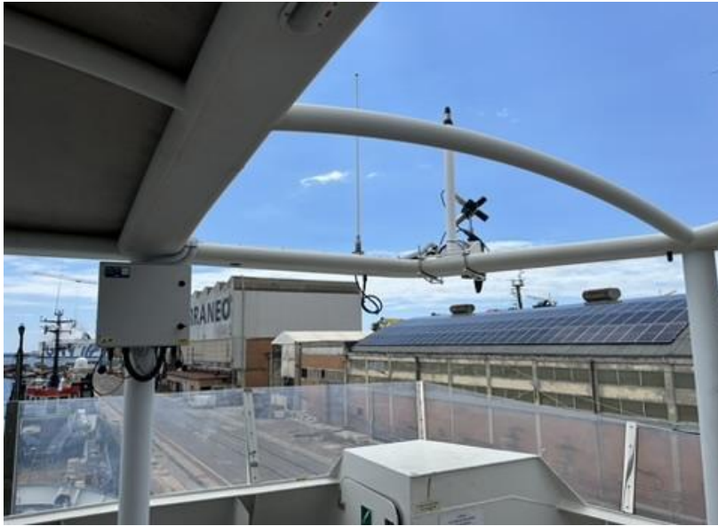
Figure 4. So-Rad system installed on the Observation Deck of R/V Gaia Blu, showing sensor positioning for radiometric measurements.
