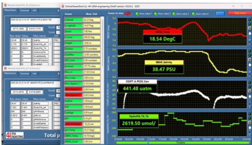
Figure 2. View of the FerryBox control panel with real-time display of the acquired parameters.
