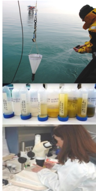
Fig. 21 - Sampling on the LTER “Acqua Alta” site and preserved samples and microscope analyses.
