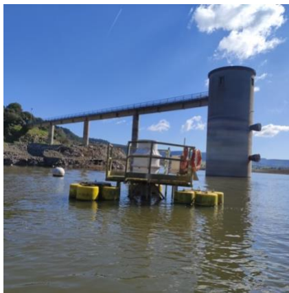
Fig. 1- Real-time remote monitoring platform in Lake Bidighinzu equipped with a multiparameter probe.
