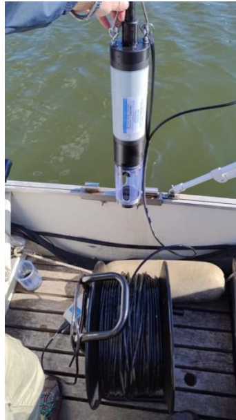
Fig. 3- Monitoring activities in Lake Bidighinzu: in situ measurements using a multiparameter probe.
