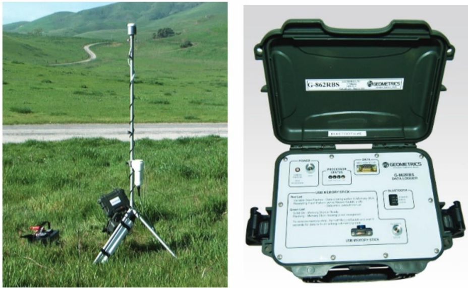
Figure 4 – Magnetic Base Station (Geometrics) to monitor and correct for diurnal variations in the magnetic field.
