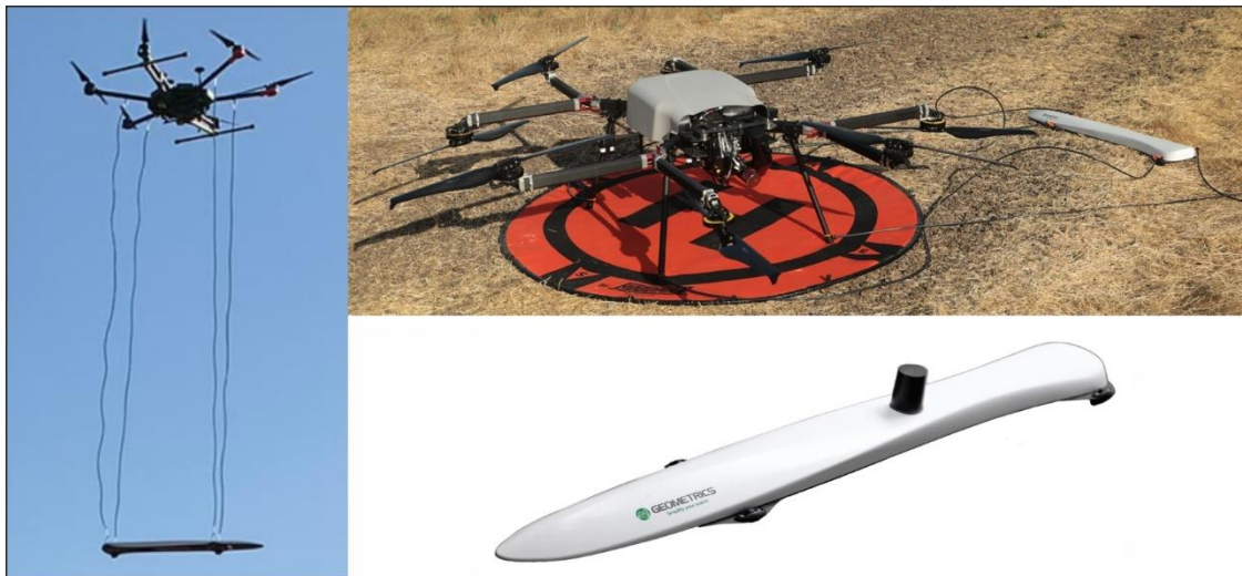
Figure 5 – Aeromagnetic drone for ultra-high resolution surveying.
