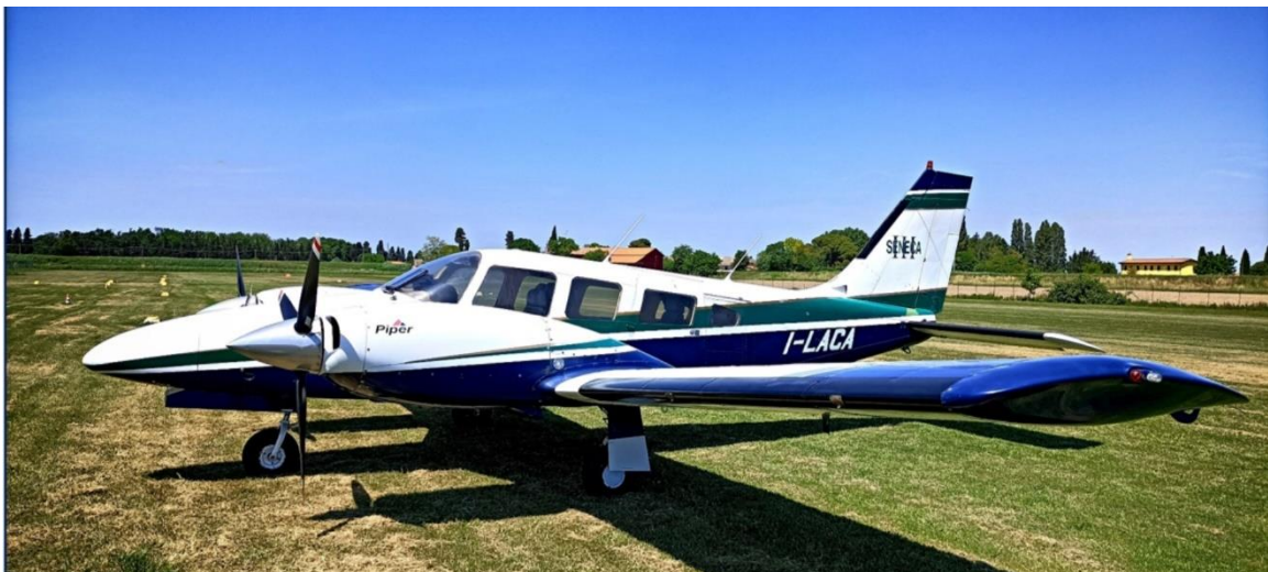
Figure 2 – The OGS fixed wing airborne platform (a Piper Seneca III), which is currently part of the remote sensing infrastructures within EUFAR.
