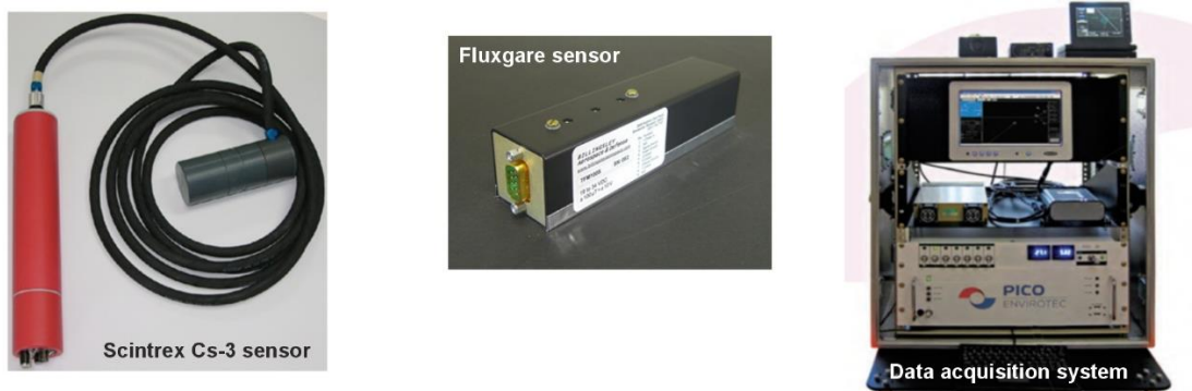
Figure 3 – Aeromagnetic sensors and data acquisition system.
