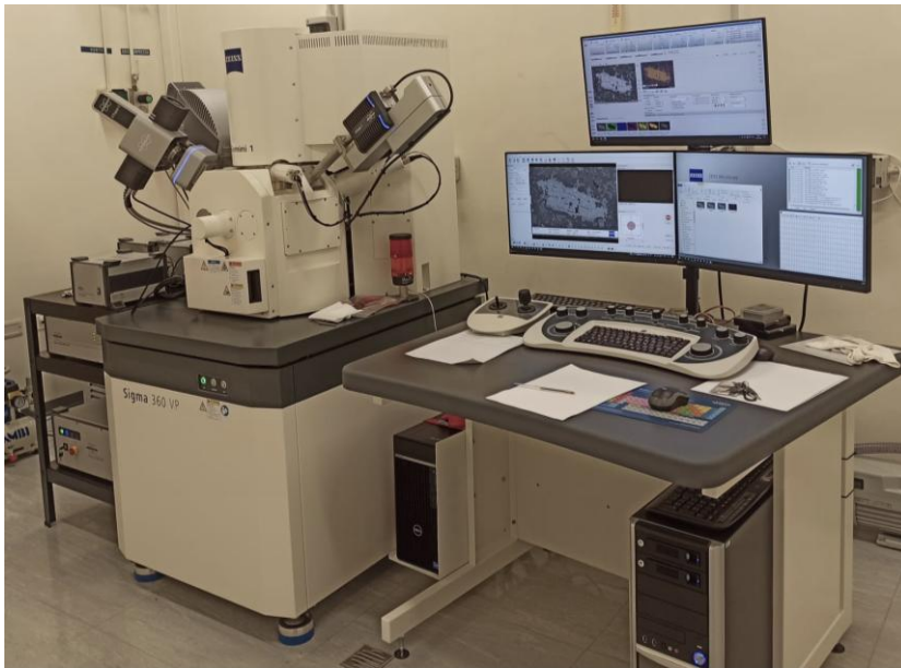
Figure 38. The high-performance Field Emission Scanning Electron Microscope (FE-SEM) installed at IGG-CNR in Pisa.
