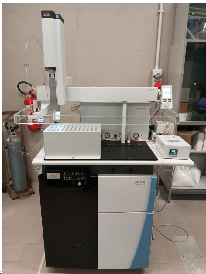
Figure 36. Delta Q, Gas Bench plus with triplus RSH autosampler installed at IGG-CNR.
