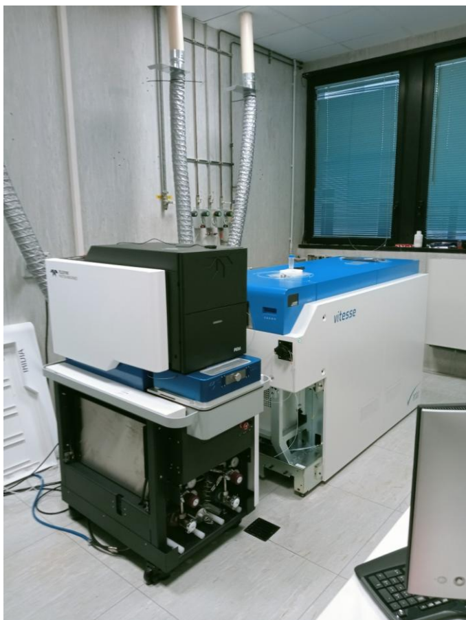
Figure 37. The LA-ICP-TOF-MS instrumentation installed at IGG-CNR in Pisa.
