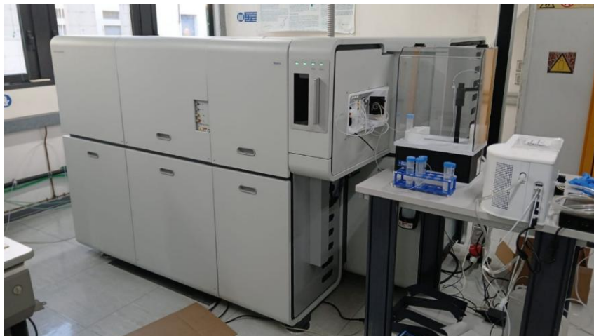
Figure 33. The new Laser Ablation (LA) - MC-ICP-MS Thermo Scientific Neoma was installed in January 2025.
